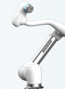
M1013 Payload 10kg Reach 1300mm
