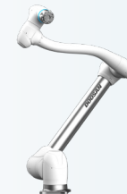
M0617 Payload 6kg Reach 1700mm
