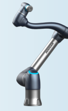
H2017 Payload 20kg Reach 1700mm
