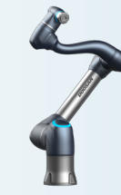
H2515 Payload 25kg Reach 1500mm
